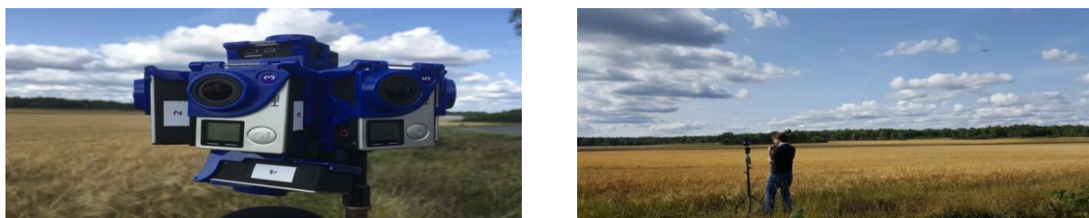
Figure 9.4 – Setup for 360 degree video recordings of the environment and the aircraft movements
