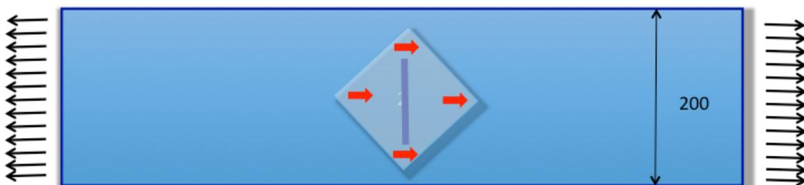
**Figure 3.** Plate with a bonded repair patch. Red arrow are sensors position
