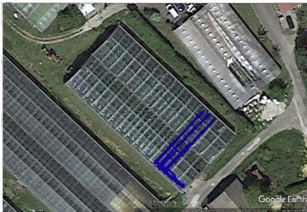
Figure 7. Google Earth plot of GPS+GAL L1/L2/E5AltBOC PPP Solution from MSP3 for Test 3 Dynamic
