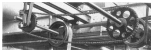
FIG. 32.—Shafting to Shafting by Roller Chain.
