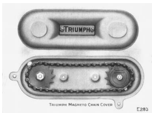
FIG. 31.—Motor Cycle Magneto Drive (Roller Chain).
