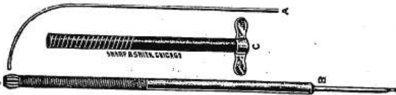
Fig. I. Ingals' Pilot Burr; two-third size. A, pilot; B, burr; C, shield.
