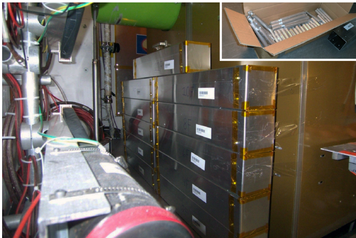
Figure 17: MoEDAL's prototype Magnetic Monopole Trapper (MMT) installed in the LHCb cavern. Each box contains several bars of aluminium (see inset image, top-right) that are later removed from the cavern and scanned using a SQUID to identify trapped magnetic monopoles. Image credit: R. Soluk/The MoEDAL Collaboration ; please contact them regarding licensing/re-use of this image.
