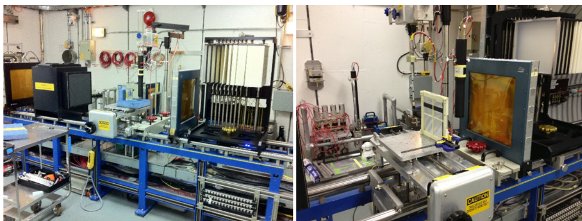
Figure 23: MoEDAL NTD samples being exposed to a heavy ion test beam at the NASA Space Radiation Laboratory (SRL), Brookhaven National Laboratory (BNL). Exposing NTD plastic to heavy ions from test beams allows us to see what monopole-like signals might look like and put our analysis procedures through their paces. Image credit: R. Soluk/the MoEDAL Collaboration; please contact them regarding licensing/re-use of this image.
