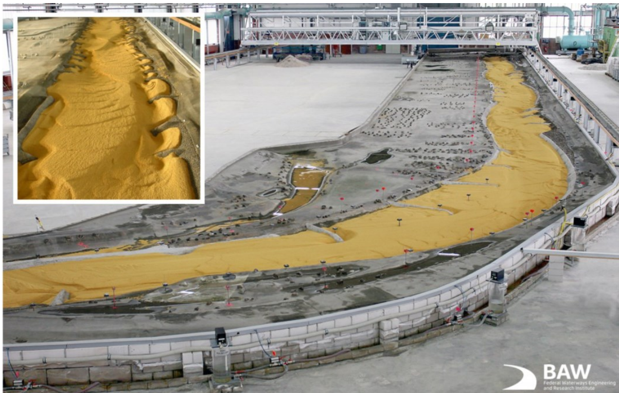
Figure 1 - Illustration of a hydraulic scaled model investigating the morphological response of a river to various hydrographs - the model of the Oder at Hohenwutzen at the Federal Waterways Engineering and Research Institute (BAW) in Germany (Henning et al. 2008). The model is built with a horizontal length scale of 1:100 and a vertical length scale of 1:40, thus with a distortion of 2.5. The full length of the model is 80 m, or 8 km in nature. The model bed is made of solid banks with groins and dams and the movable lightweight sediments are a polystyrene plastic granulate.
