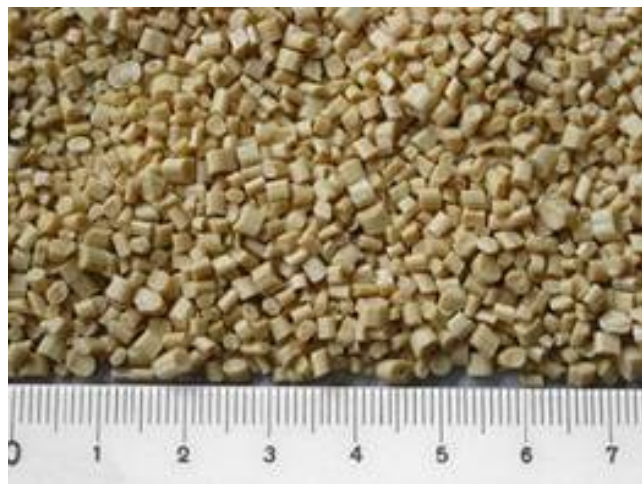
Figure 5 - Polystyrene sediments ( d_m = 2.1 mm, d_{60}/d_{10} = 2.0 , \rho_s = 1055 kg/m 3 ) used in the Oder model shown in Figure 1.
