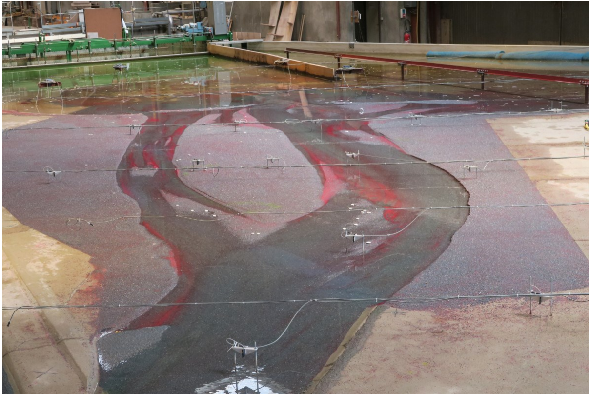
Figure 12 - Physical scale model of the Rhone delta in Lake Geneva-courtesy Artelia (see Bollaert et al. 2017)
