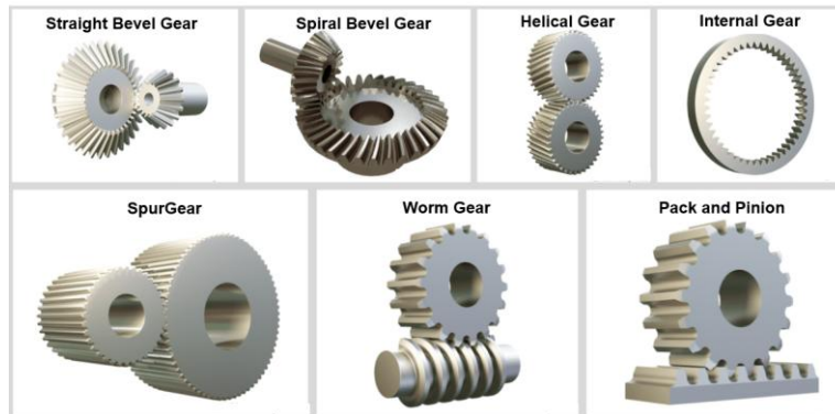
Figure 42. Types of common gears [34]
