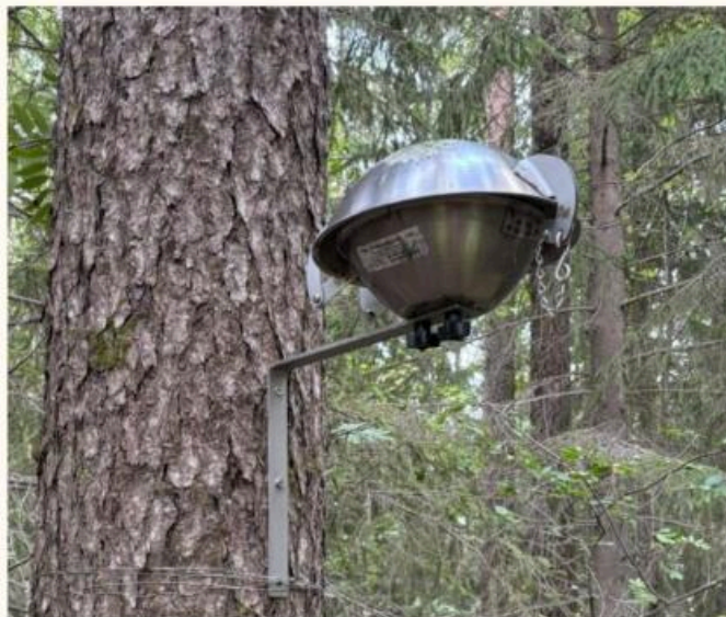
Passive dust sampler installed at the Ihalainen mining site.
