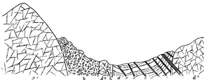
FIG. 54.—Section from Beinn Dearg to Beinn an Dubhaich, Skye. aa , Lower Silurian limestone; bb , volcanic agglomerate; ccc , basalt-dykes older than granophyre; d 1 , granophyre of Beinn Dearg; d 2 , granophyre in the agglomerate neck; d 3 , granophyre of Beinn an Dubhaich; e , basalt-dyke younger than granophyre.
