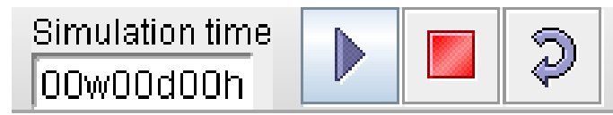
Figure 2. JASS basic counter and controls: start, stop and reset (in that order). The stop button pauses the simulation. It will continue at the same time when the start button is clicked again. The reset button resets the system to the initial conditions.
