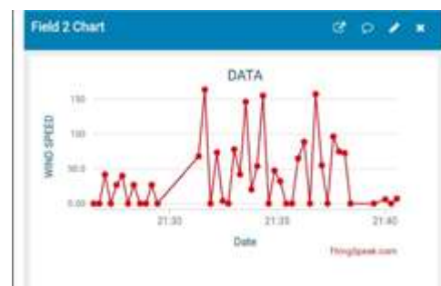
Fig. 2. Wind speed fluctuations recorded over time, used as input data for machine learning-based wind energy forecasting.
