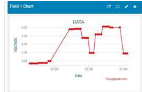
Fig. 1. Real-time voltage variation of the microgrid system obtained from sensor data and visualized using ThingSpeak platform
