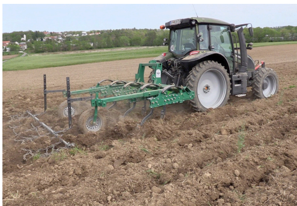
Figure 3. Preparation of the ridges with the Turiel Dammsystem
