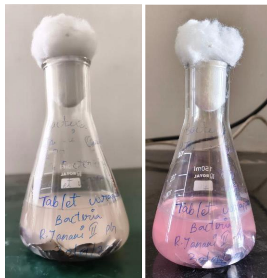
Fig. 2 Degradation of Tablet Wrapper by Pseudomonas putida
