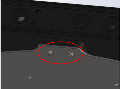
Slide the washers over the M2x8 bolts and mount the camera to the top plate using the spacer.
