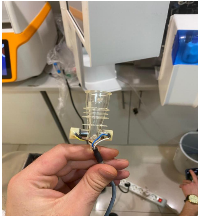
Figure 3. Replacement WBC/HGB chamber in Hematology analyzer.
