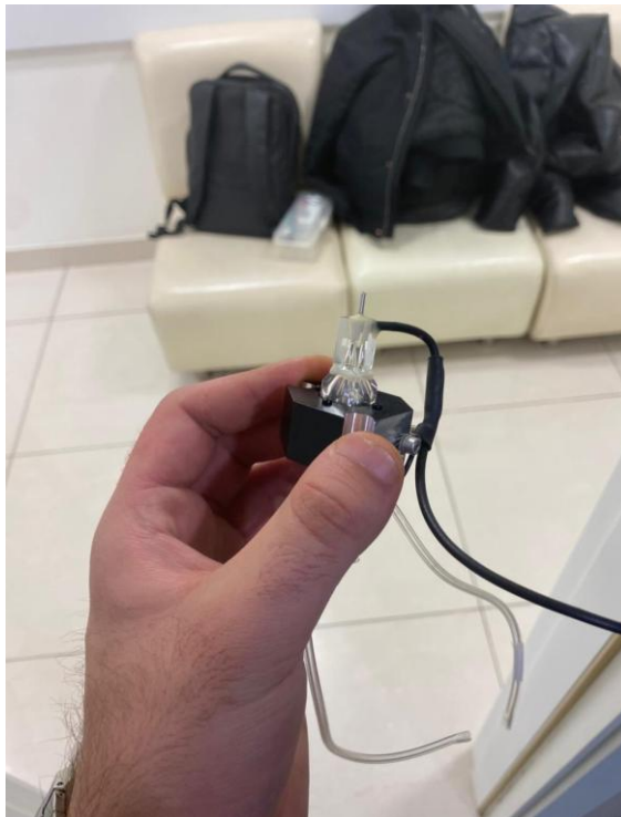
Figure 4. Flow cell in Hematology analyzer.
