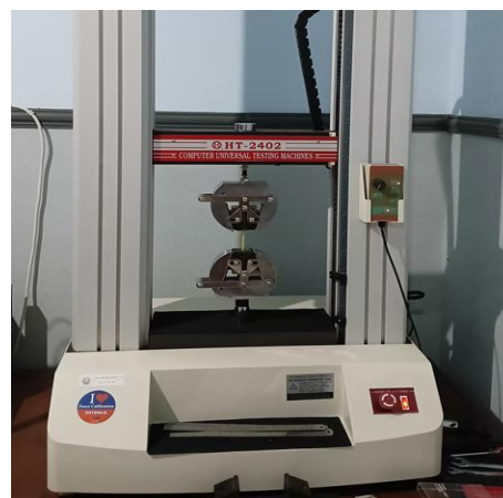
Fig. 3: Tensile test setup (HT-2402 UTM)
