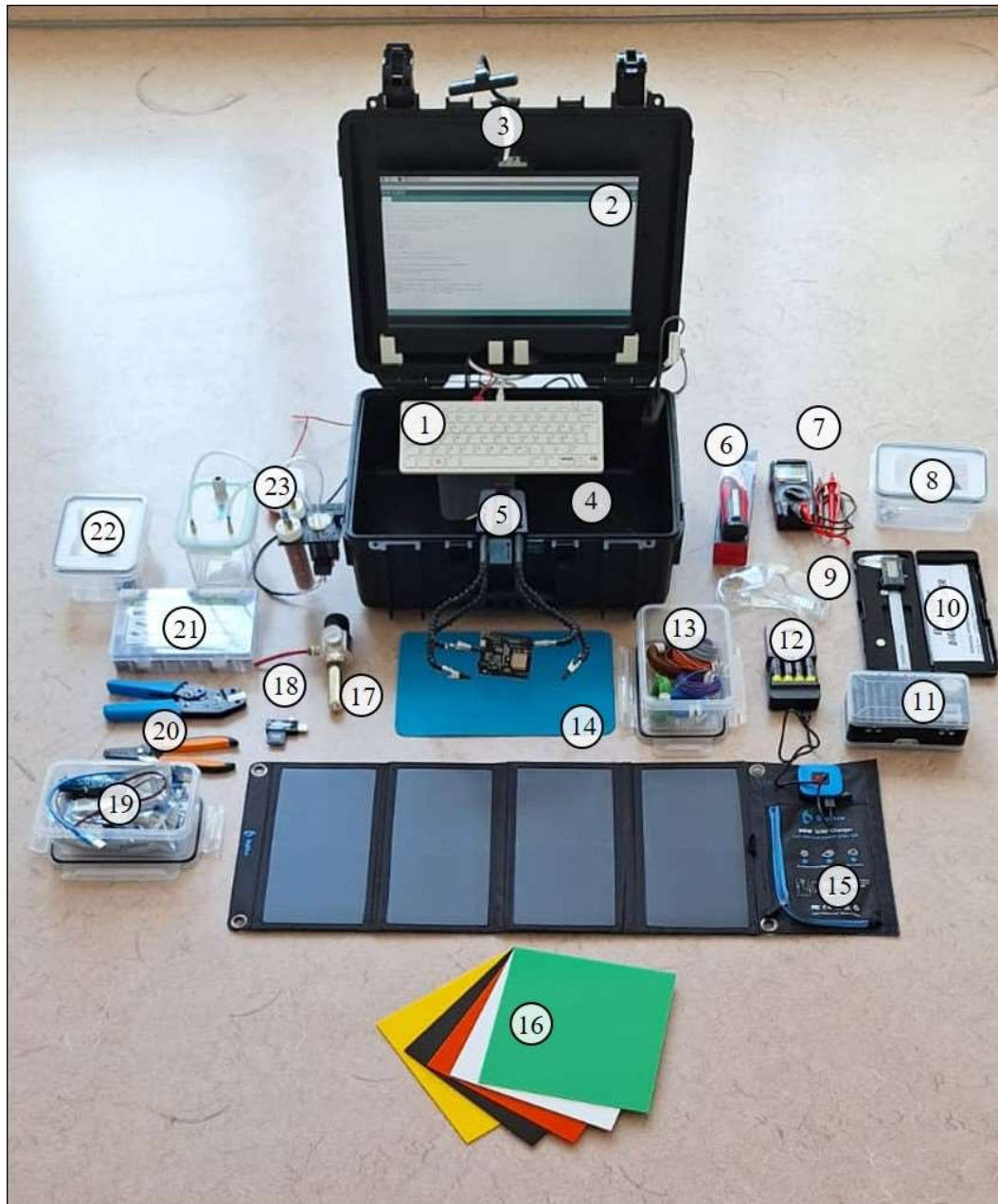
Fig. 2.1.4: Overview of the "Lab on Wheels" maker space assembled within a weatherproof outdoor box. It contains: (1 - 2) Pi400 and screen for programming of microcontroller, (3) a solar chargeable USB lamp, (4) a power bank to supply power to the Pi400 and screen, (5) a third hand for easy soldering, (6) a battery powered solder iron, (7) a multimeter to check voltage and connectivity, (8) A USB chargeable rotary tool for small grinding and drilling tasks, (9) security goggles, (10) a digital caliper, (11) a fine mechanic set with tweezers and a multi-bit screwdriver set, (12) a USB NiMh battery charger, (13) a wire set, (14) a solder mat, (15) a 28W foldable solar panel to charge the power bank, rotary tool, lamp, and battery charger, (16) 5 colored acrylic plates as transfer standard to calibrate the low cost NDVI sensor, (17) a brewery valve and CO 2 /N 2 O cartridge for low cost sensor validation, (18) a SD(MicroSD) card reader, (19) diverse microelectronic components as well as a USB type-B-cable and FTDI
