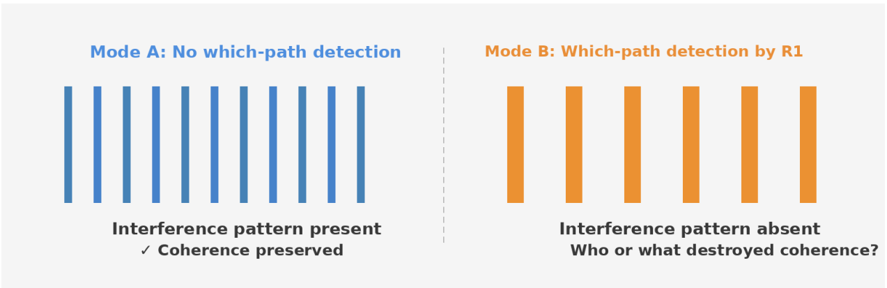
Figure 2: Schematic comparison of the patterns expected on the screen for the two modes of operation. Mode A (left): without which-path detection, interference is expected. Mode B (right): with which-path detection by R1, the question is whether the loss of interference requires a conscious observer.
