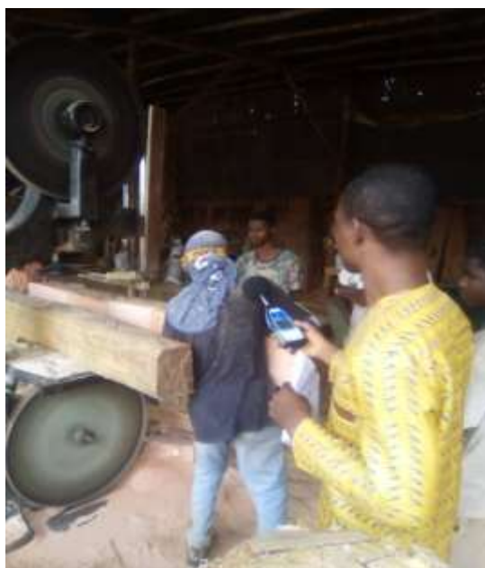
Photo 7: Measurement of equivalent continuous sound pressure levels L_{p,A,eqT}
