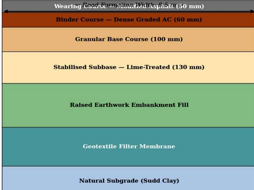
Figure 3: Proposed Flood-Resilient Road Cross-Section for Sudd Wetland conditions, showing layer sequence from subgrade through wearing course with geotextile membrane and raised embankment.
