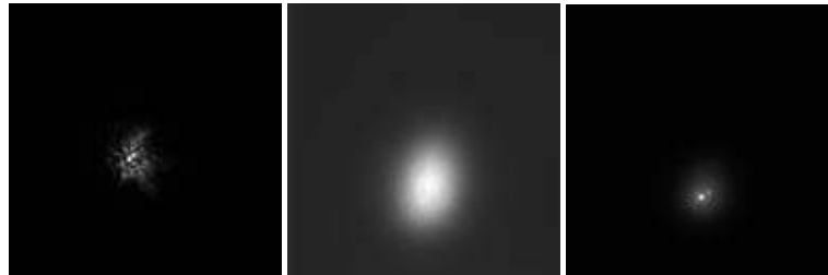
Fig. 5. Left: a 30ms exposure. Centre: natural seeing. Right: 1% of 4,000 aligned and averaged images.
