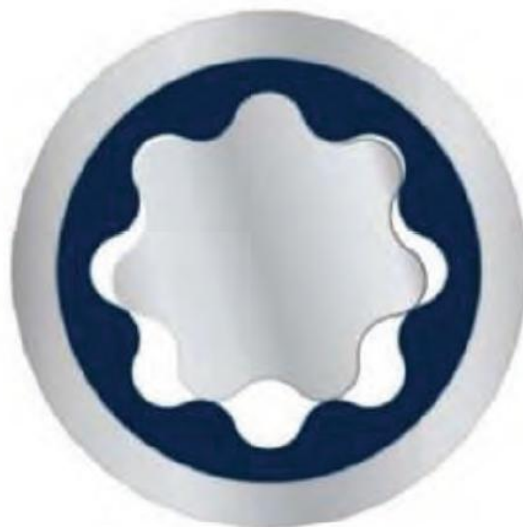
Figure 1: Cross-section of a 7/8 power section: 1 – stator, 2 – rotor, 3 – elastomer [7].
