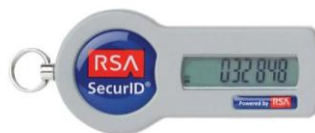
Figure 1.2: Example of an RSA SecurID hardware authentication token.
