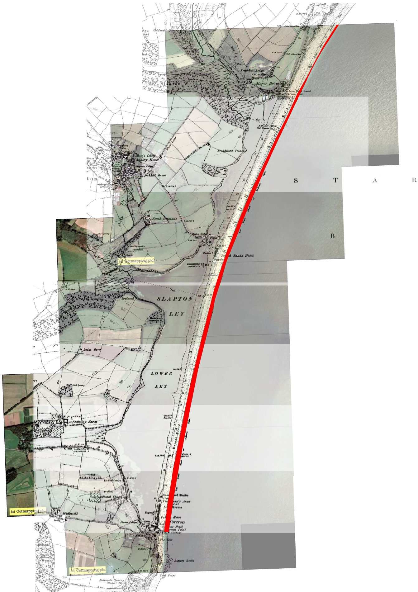
Fig. 3.6 Shoreline recession at Slapton between 1890 (map overlay) and the present day (aerial photo). The approximate recession in low tide shoreline is marked in red. Based on a figure prepared by Prof. Roland Gehrels, University of Plymouth.
