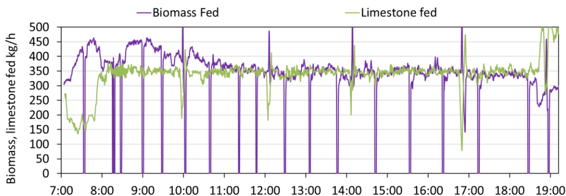
Figure A.107. Biomass and limestone feeding rates fed to the calciner reactor (Experiment 06/03/24).
