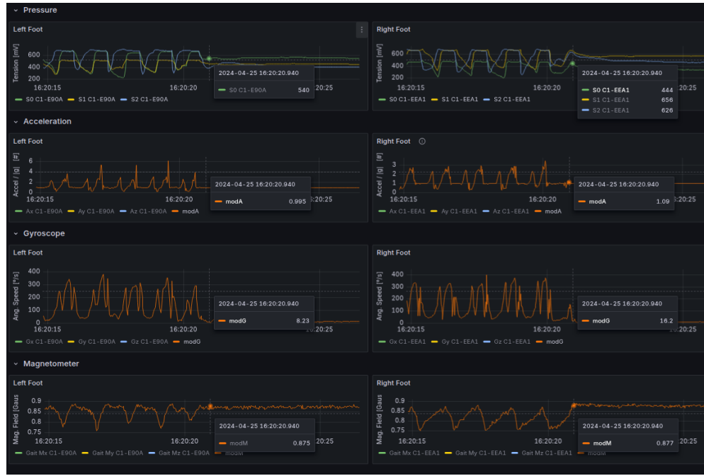
Fig. 2 Data collected from Sesonria Inc trademark socks. Pressure but also acceleration, rotations from gyroscopes and magnetometer signals have been recorded in an InfluxDB engine.
