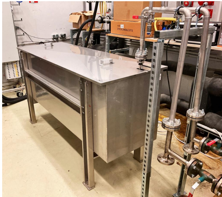
Figure 12: Latent heat storage (not insulated) connected to a thermostat in AIT's thermal storage laboratory
