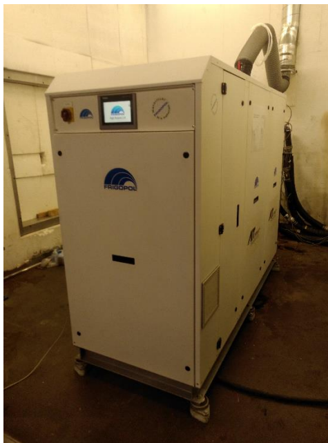
Figure 3: High-temperature heat pump in a climate chamber of AIT's heat pump laboratory
