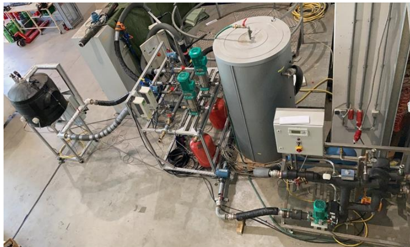
Figure 22: Setup in the AIT heat pump laboratory with main components: Boiler (left, black), storage tank (centre, grey), three circulation pumps (green) with frequency converters, flow meters (blue), expansion vessels (red), tubes and pipes almost completely insulated.
