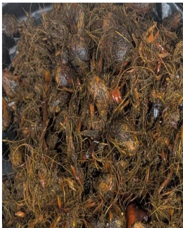
(c) Sample of digested palm fruits after being process in the digestion machine
