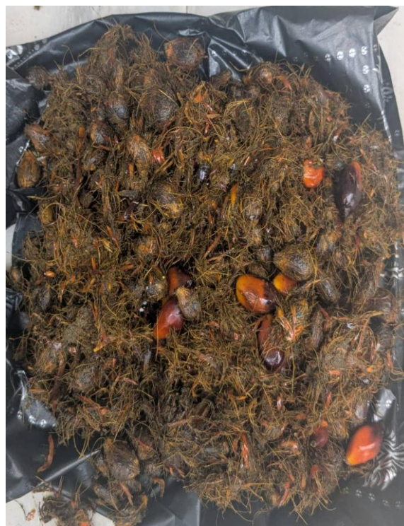
(b) Sample of unseparated palm fruits after being process in the digestion machine
