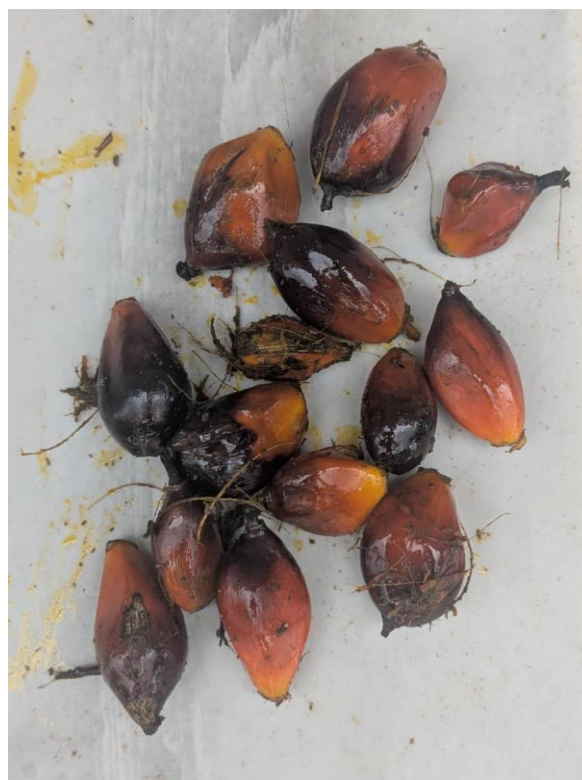
(d) Sample of undigested palm fruits after being process in the digestion machine
