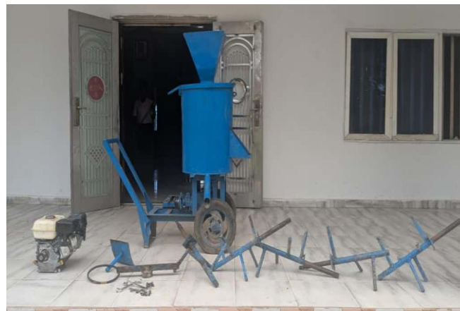
Figure 3.2 shows the pictorial view of the component part of the developed palm fruit digestion machine
