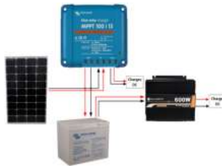
Figure 1: Photovoltaic system wiring
