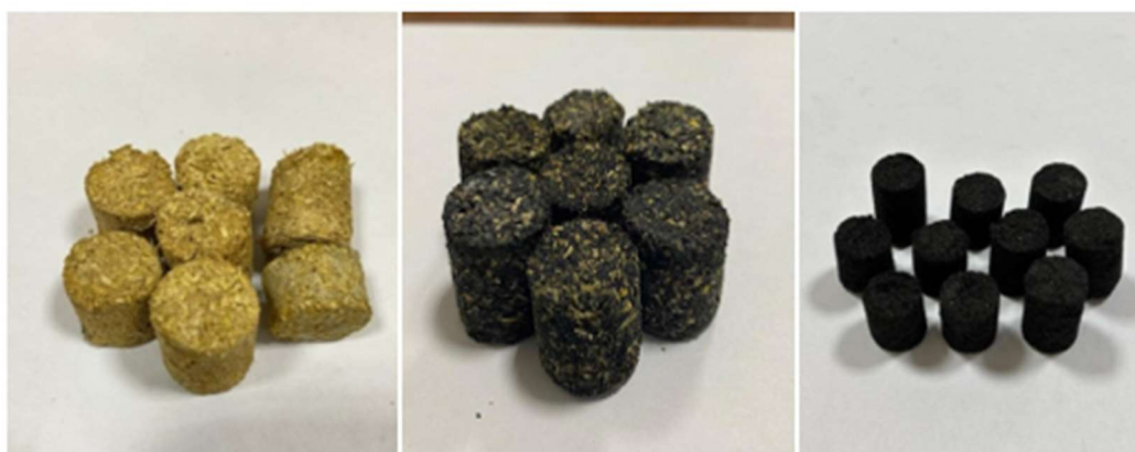
Fig. 1 - a) Briquette from wheat straw; b) Briquette from a mixture of coal and biomass 50/50 c) Briquette from Shoptikol coal
