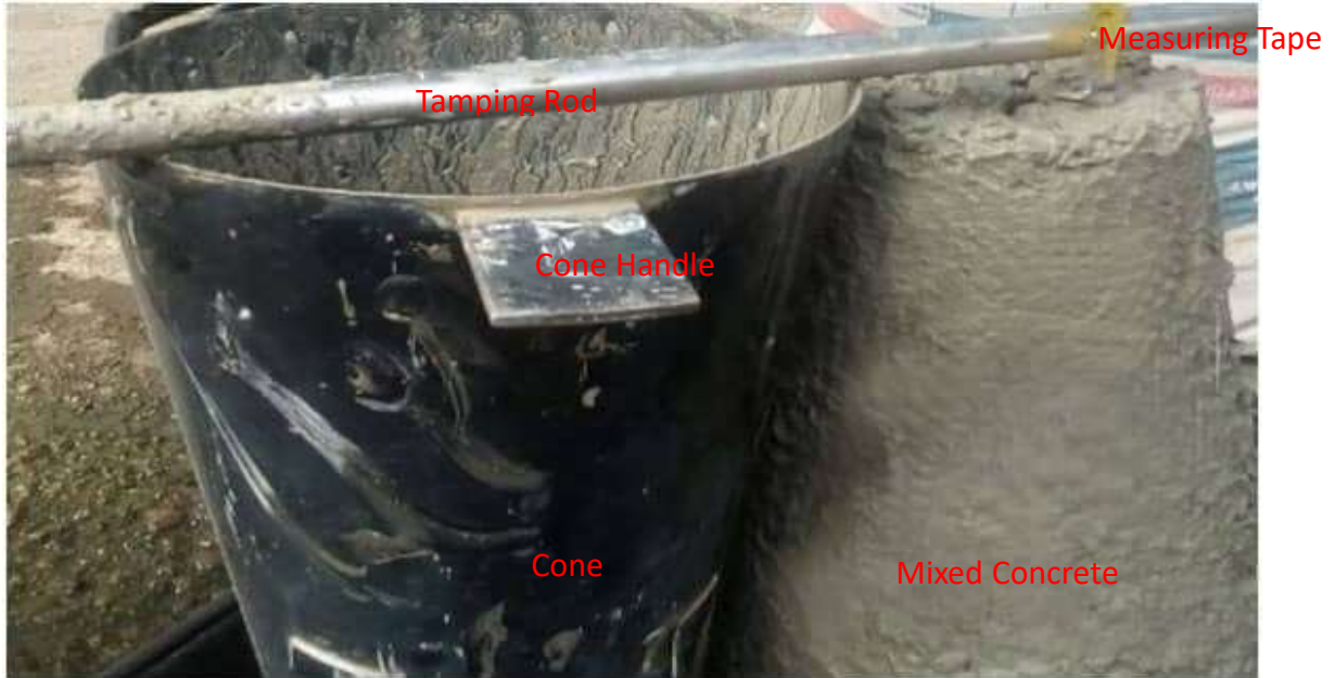
Fig. 5: Slump measurement
