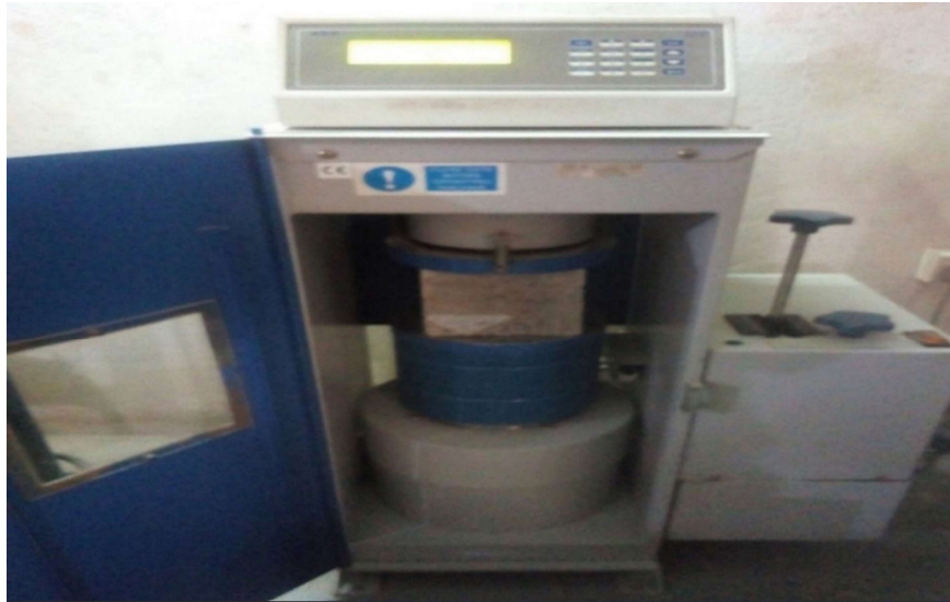
Fig. 6: Compression testing Machine with concrete cube
