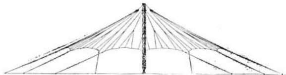
FIG. 2.—DIAGRAM OF TOWER AND ANTENNA.
