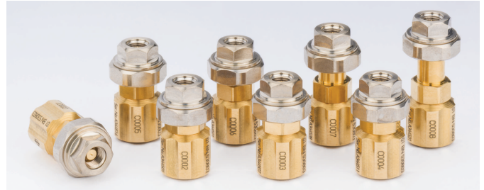
Fig. 1. Primary offset shorts (C2–C8, standing) with offset lengths between 1.153 and 10.000 mm. A flush short (C1, lying) is used as verification.
