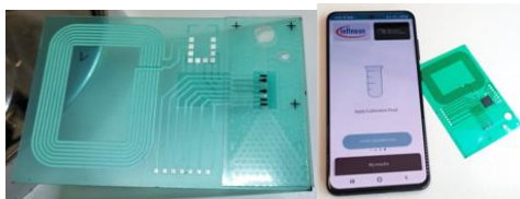
Figure 1: left: sensor sheet with bonded microfluidics; right: sensor card with smartphone
