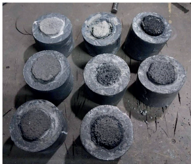
Fig. 4.16 Samples: a – pattern blocks; b – casting bushes
