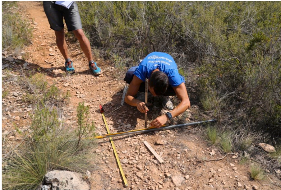
Fig. 6. Example of trail erosion measurement using the cross-sectional-area method. Measurements here are being made in the Serra Grossa El Portalet trail, Eastern Iberian Peninsula.
