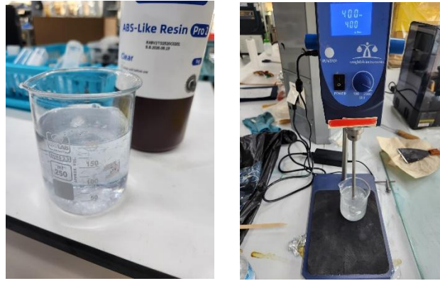
Figure 1. Mixing process of the fiber-reinforced ABS-like resin performed at 400 rpm for 5 minutes.
