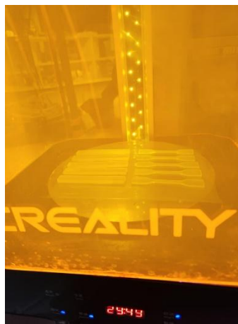
Figure 4. Curing process at 405 nm wavelength for 180 minutes.
