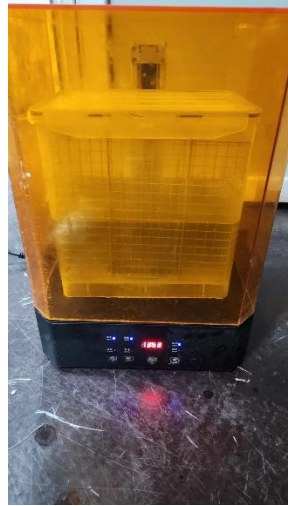
Figure 3. Washing of the 3D printed specimens in an isopropyl alcohol (IPA) bath for 30 minutes to remove uncured resin.
