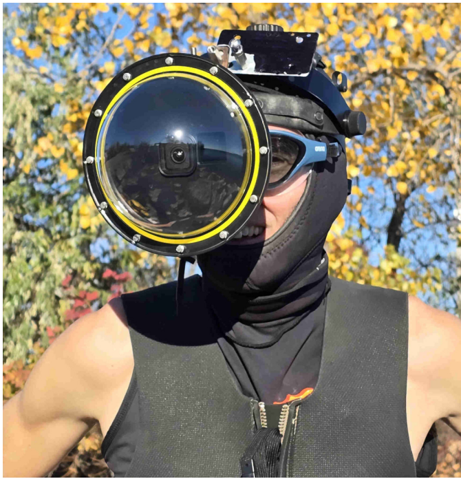
Fig. 5: Prof. Steve Mann with his Headome™ invention. The Headome provides underwater eyesight that perfectly matches the refractive index above and below the water, without requiring any special contact lenses as were required with previous similar technologies invented by others.
