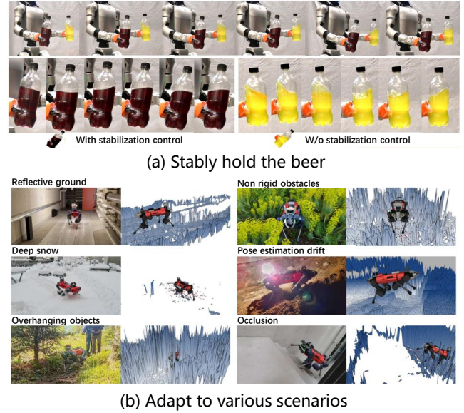
Fig. 21 Precise tasks, like (a) steadily holding the beer [363], demand accurate physical prediction, which requires a specialist world model. In contrast, (b) completing diverse tasks in complex environments [54] calls for a generalist with stronger generalization.
