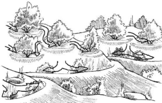
Fig A.3.2.1-2 A series of swales and bunds.
