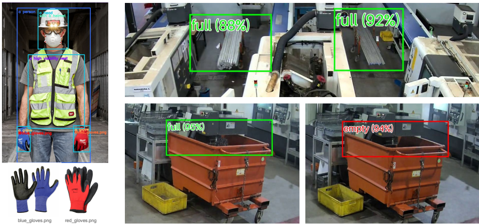
Figure 5.3: Application of the OVD component in the Pilot 2 industrial scenario. (Left) PPE detection using a mixed textual-visual and hierarchical vocabulary. (Right) Container status detection using visual vocabularies to classify material and waste containers.
