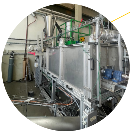
Slow pyrolysis auger reactor
