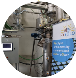
Fast pyrolysis fluidized bed reactor
