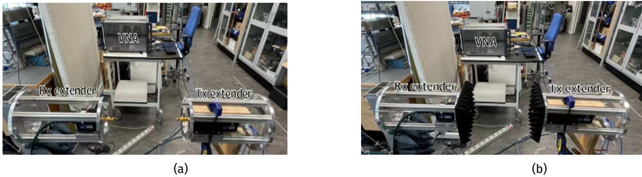
Figure 3: The photos of the channel measurement setup: a) Without absorber; b) With absorber
