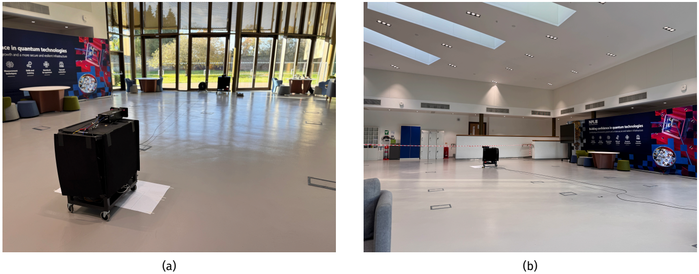
Figure 54: Atrium measurement location with (a) receive trolley located in position Rx2 and (b) the receive measurement trolley from the perspective of the transmit antenna
