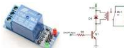
Figure 2. Relay shape and symbol [6]
