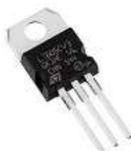
Figure 7. LM7805 Regulator IC [14]
