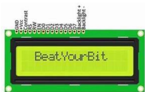
Figure 4. Pins on 16x2 LCD[10]
