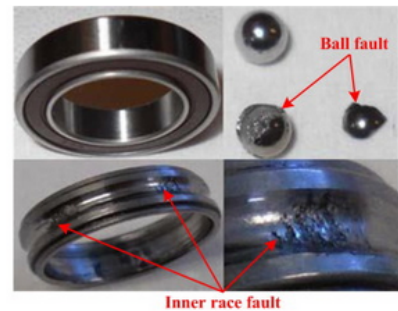
Figure 19: Different faults of rolling element bearings [45].
