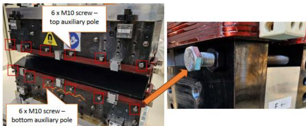
Figure 14: Auxiliary pole horizontal adjustment.
