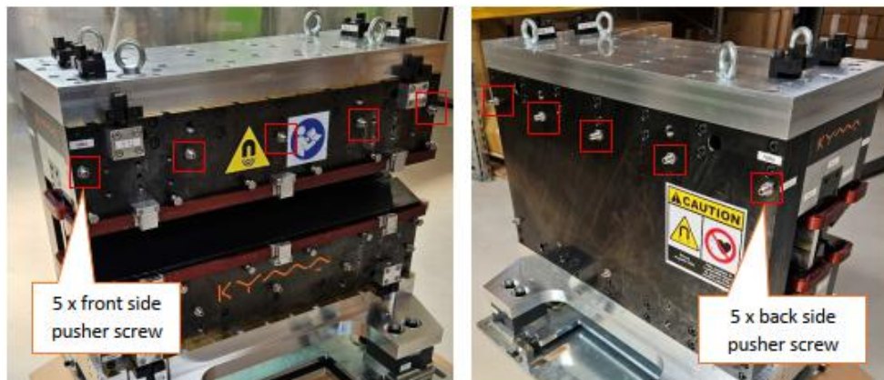
Figure 10: Top main pole horizontal adjustment.
