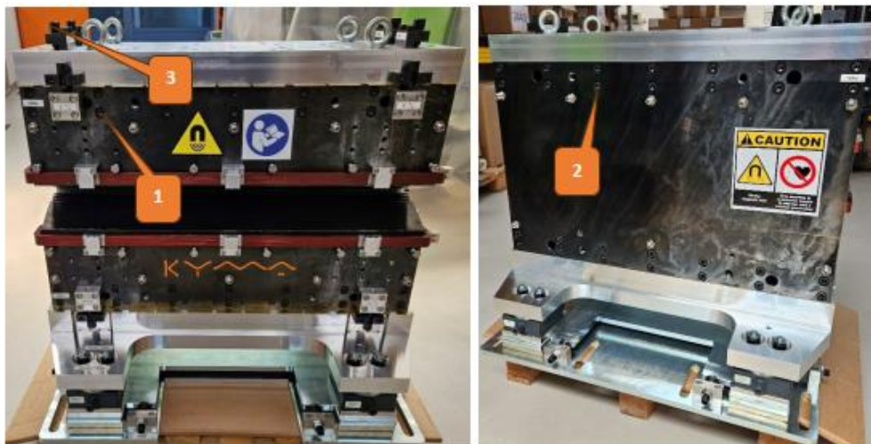
Figure 28: Slightly loosen the screws (1) and (2) prior to main pole vertical adjustment.
