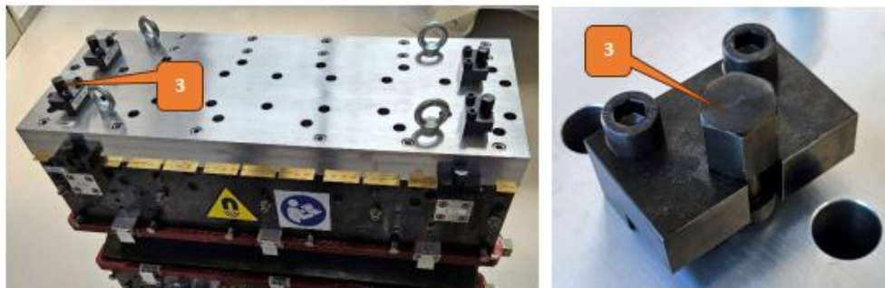
Figure 29: Rotate the adjustment screws (3) in the clockwise direction to lift the top main pole.
