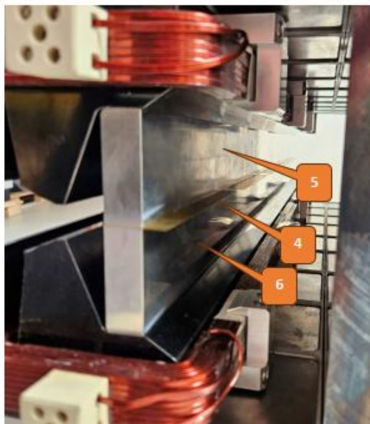
Figure 30: Insert / remove brass shims (4) between the main pole spacers (5) (6).
