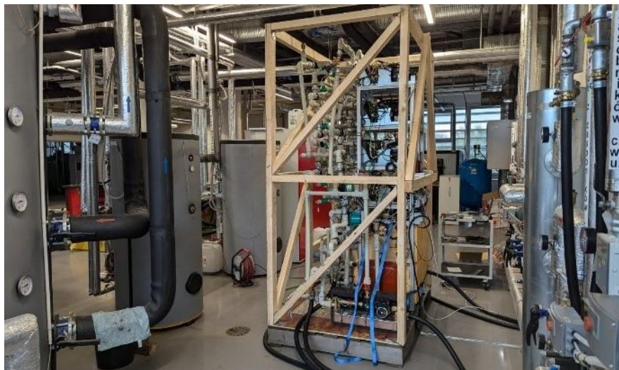
Figure 6 The modular heat pump connected to KEZO system.
