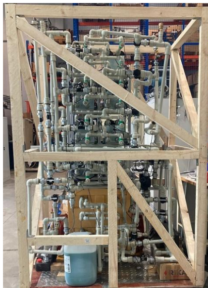
Figure 6: The modular Heat Pump developed by OCHSNER.
