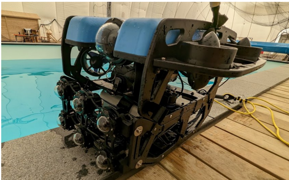
Figure 3.5 | BlueROV2 with adjustable multi-camera rig payload integrated and tested in DTU's Autonomous Systems Testing Arena.
