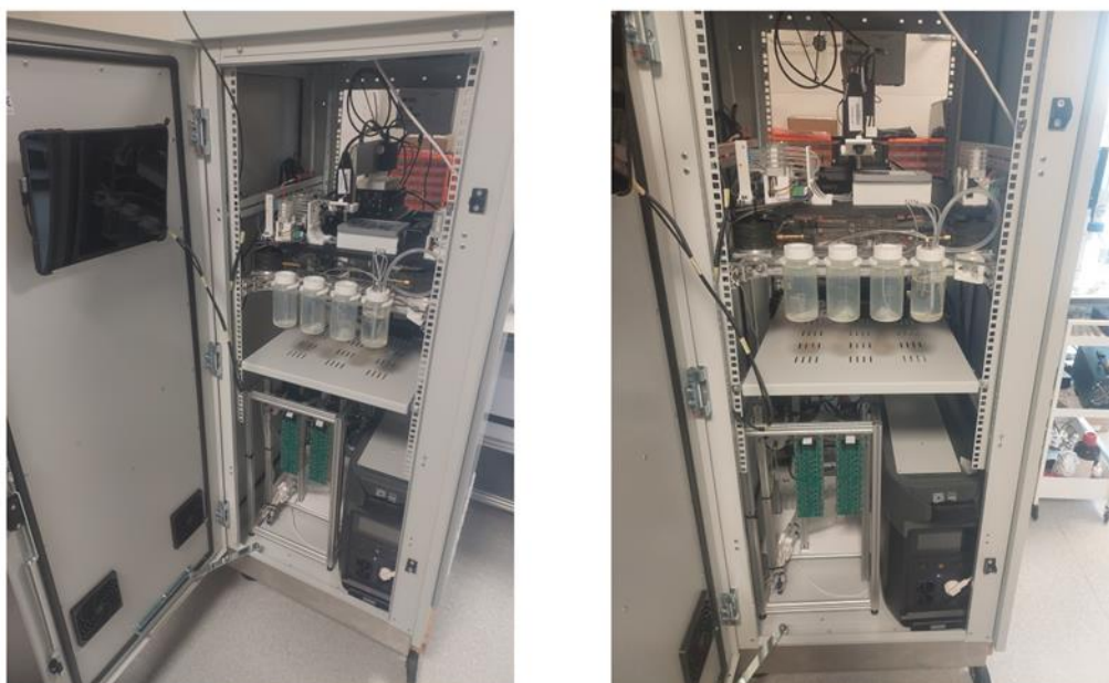
Figure 3 Images of the multi-analyte monitoring platform used for metals, microplastics and CECs detection (from deliverable 2.5).
