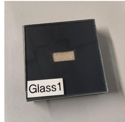
FIGURE 5: SAND PARTICLES INSIDE ASSEMBLY OF CRUCIBLE AND GLASS TO MEASURE THE OPTICAL PROPERTIES IN THE PERKIN-LAMBDA SPECTROMETER.
