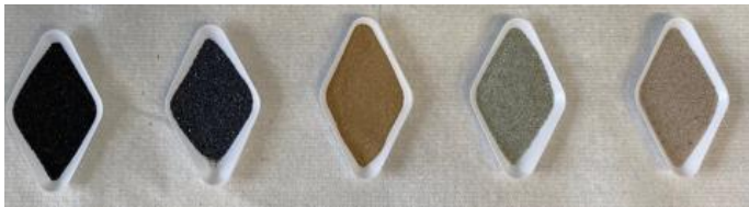
FIGURE 1: POSSIBLE PARTICLE HEAT CARRIERS FOR PYSOLO PROCESS (FROM LEFT TO RIGHT: BAUXITE, SiC, MgO, OLIVINE AND SAND).
